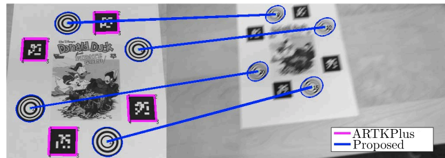
Figure 9. Detection and matching of fiducial across two images under challenging shooting conditions: the left image is correctly focused contrary to the right image which is acquired by a fast moving camera which generates motion blur. The ARToolkitPlus system correctly detects and identifies its markers (surrounded in magenta) only in the sharp (left) image whereas no one is detected in the blurred view. The proposed system correctly detects and identifies the imaged markers in the two images.
