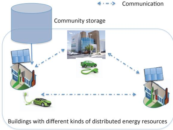
Fig. 2. Distributed energy generation and storage with mobility for enhanced resilience during emergencies
