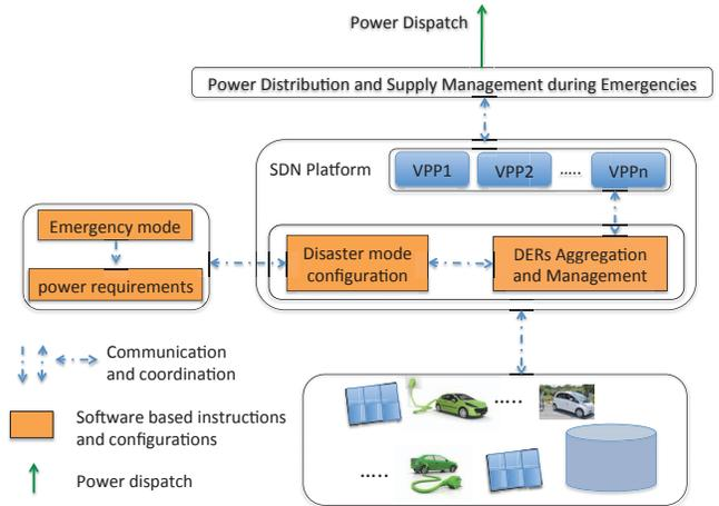
Fig. 3. SDN coordinated distributed energy generation, storage, aggregation and dispatch
