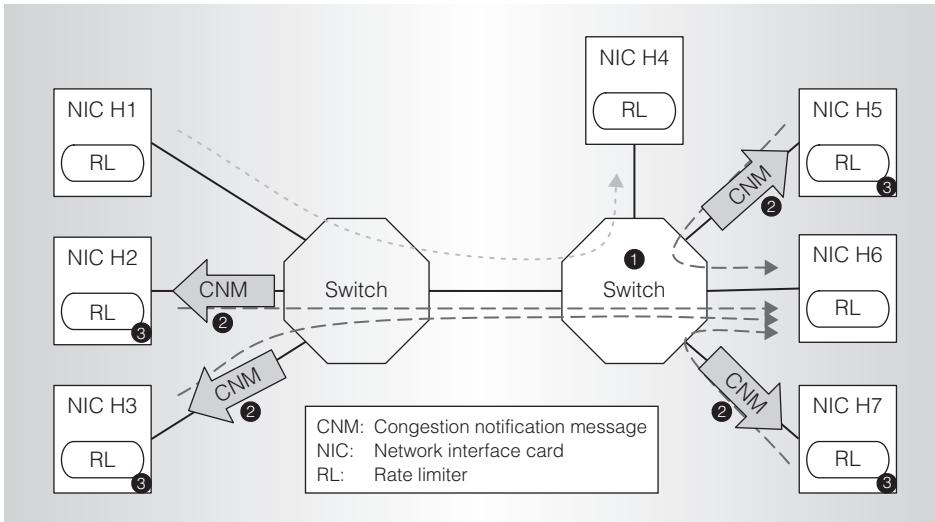
Figure 2. Quantized congestion notification protocol with the congestion point (1), congestion notification message (2), and rate limiter (3).
