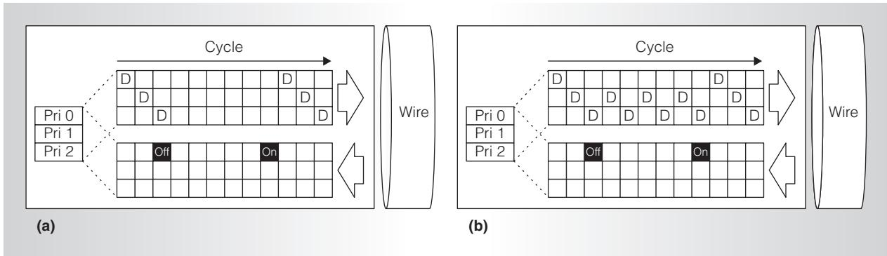
Figure 1. The effect of per-link (a) and per-priority (b) flow control on link activity. With per-link flow control, all transmission on all priorities is halted when transient congestion occurs. With per-priority flow control, only transmission on the priority where transient congestion occurs is halted.
