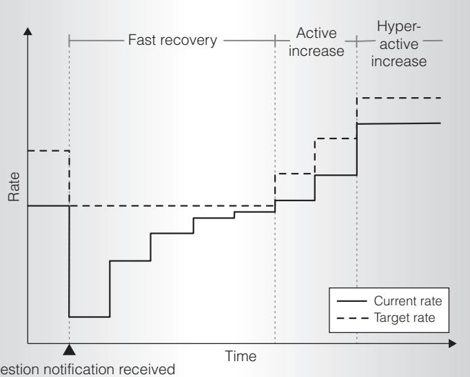
Figure 3. The process of rate decrease and rate increase at the reaction point. After a rate decrease, a new target rate is set and the rate limiter will slowly try to increase the sending rate to match the target rate. The rate increase happens in the three stages (fast recovery, active increase, and hyperactive increase), where each stage increases the rate faster than the previous one.
