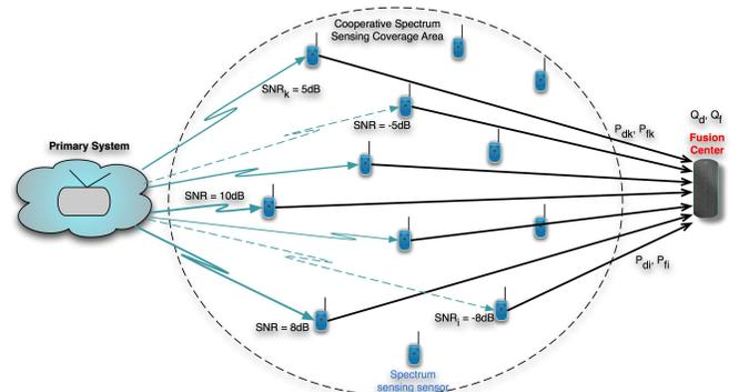
Fig. 1. Cooperative spectrum sensing model
