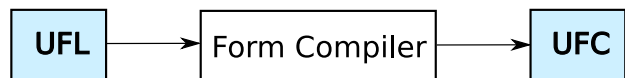
Figure 4: An abstract definition (UFL) of a finite element variational form is given as input to a form compiler, which generates UFC code as output.
