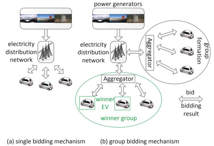
Fig. 1: The proposed group bidding mechanism in V2G networks
